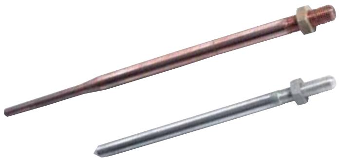
A single earth rod may not achieve the required resistance figure and several may be needed to be fitted to achieve this; their combined resistance is proportional to the reciprocal of the individual rod resistances to earth. This rule holds true as long as each rod is situated outside the resistance area of any other. To ensure this is the case, it is generally accepted that the minimum spacing between rods should not be less than their driven length.
